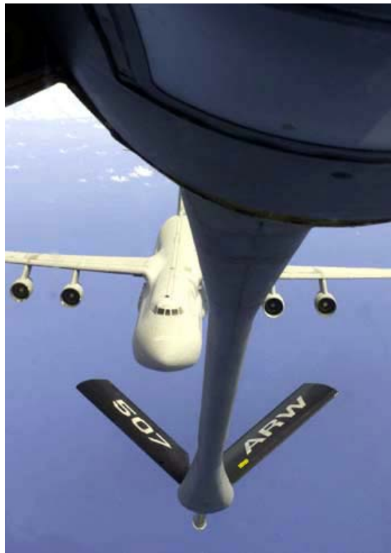
Figure 6: Lockheed C-5 Galaxy refueling by KC-135 with an Example of a Boom
